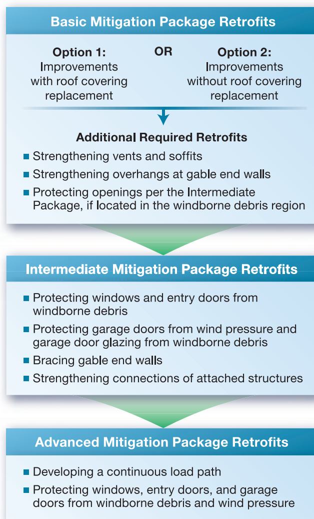
Figure 15-15. Wind Retrofit Mitigation Packages
